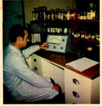
Pye Unicam meter in Tecnico's quality control lab checks the pH of a photo-resist solution used in manufacture of printed circuits. Full information on printed circuits is in survey starting page 16.
