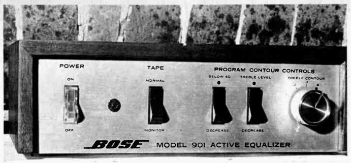
Control panel of active equaliser. The equaliser is inserted between the existing pre-amplifier and main amplifier.
