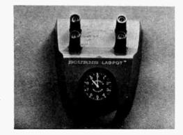
A ten-turn precision potentiometer mounted in a rugged plastic case is now available from Bourns Inc. Intended for circuit development or educational use, the units are available with a choice of analogue or digital readout.
