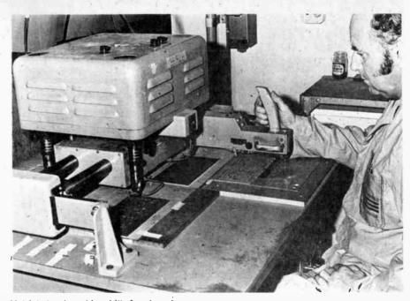
Multiple head machine drills four boards at once.
