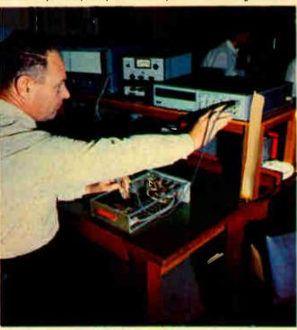
Modular construction is a feature of Natronics' Australian-made range of digital instrumentation; this frequency counter becomes 0.02% dvm by interchanging function units (test report next month).
