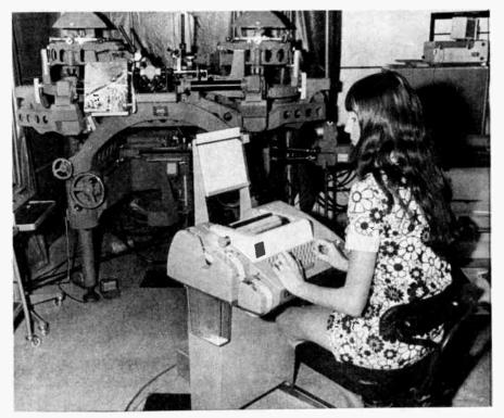
Computer terminal of Australian Aerial Mapping compares digital coordinates of scanned territory with known reference data to relate photographed stereo pairs with earth's surface.
