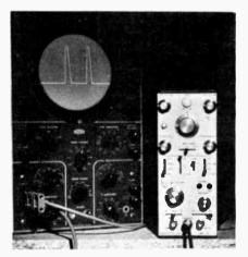
Model 610 captures a transient waveform
