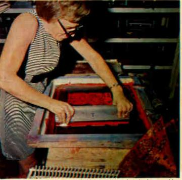
Silk screen process imprints circuit pattern onto board prior to etching.
